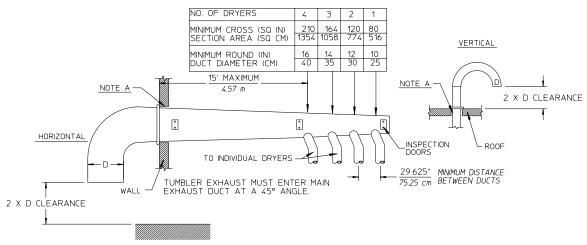
IMPORTANT: NO MORE THAN 4 DRYERS (8 TUMBLERS) CAN BE CONNECTED TO ONE COMMON DUCT (VENT).
